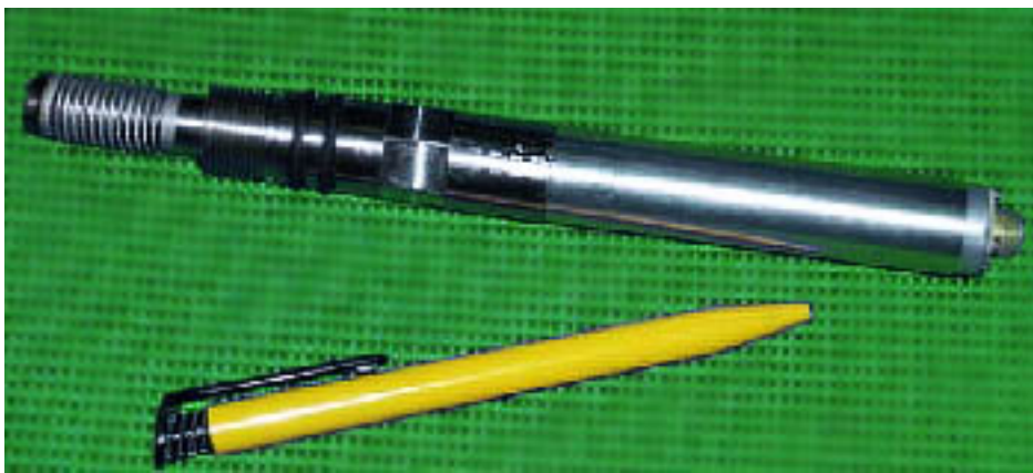
Fig. 3. Precision quartz downhole sensor PDTK-60MC
